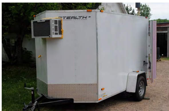
Refrigeration trailer using A/C system with CoolBot technology. Credit: EverGood Farm
